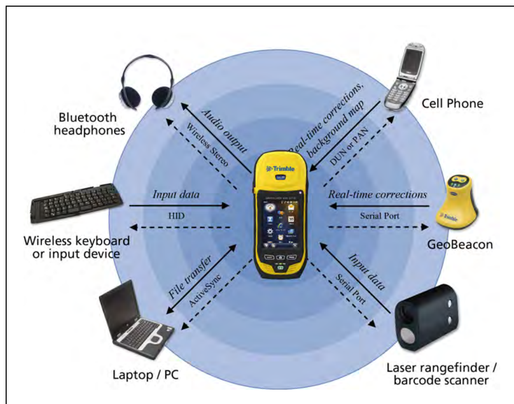
Figure 6.1 GeoExplorer 6000 series handheld Bluetooth client connections
