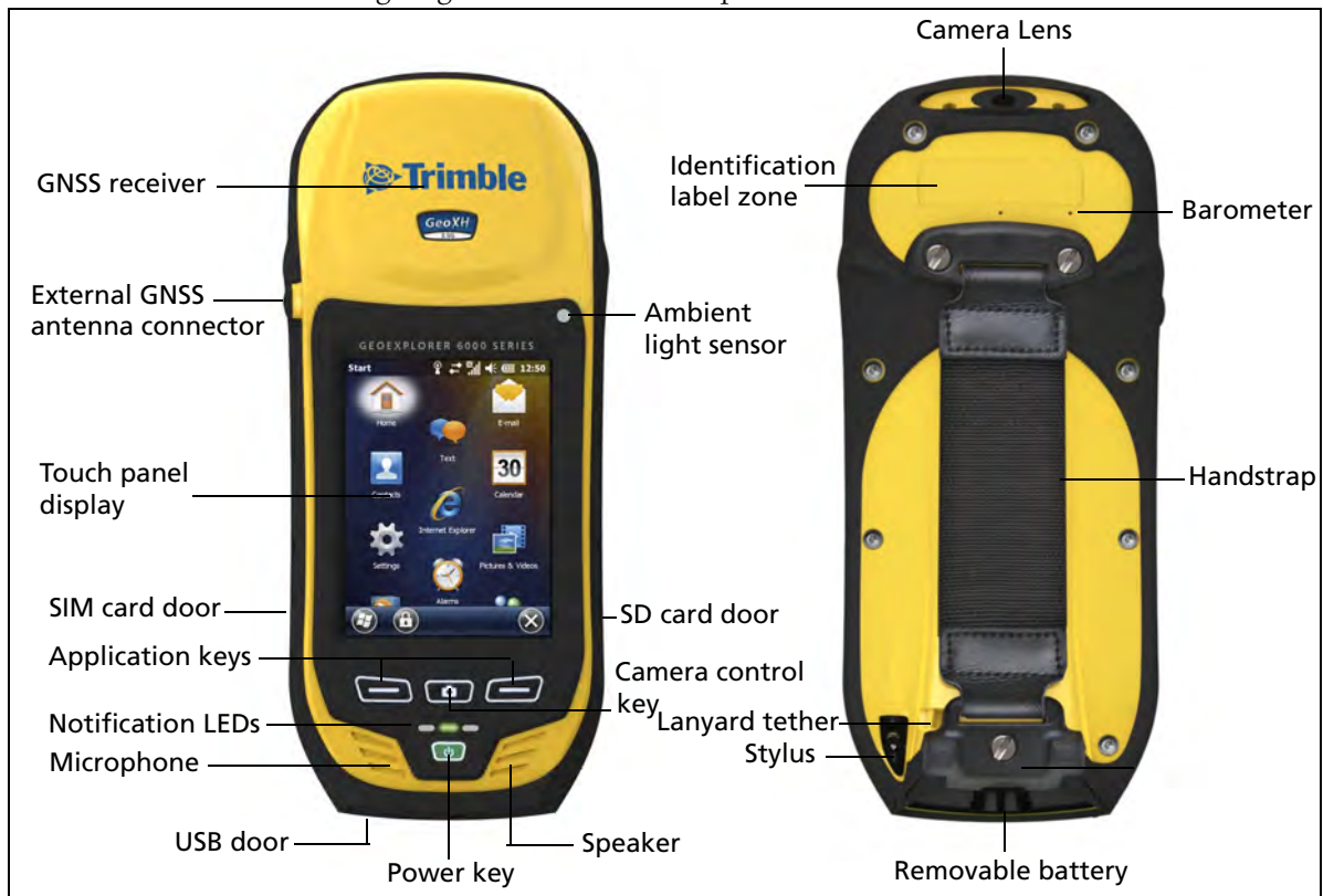
Figure 2.1 Parts of the GeoExplorer 6000 series handheld
